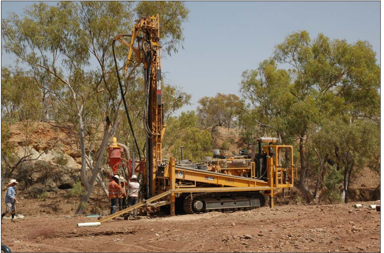
Fig 3 - RC drilling within the D-Tree JV area – September 2008.
